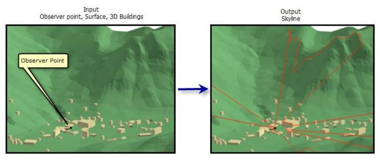
Mapping the horizon around each pixel (both from terrain and urban orography)
